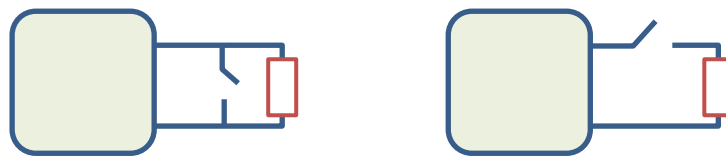
Abb. 1. Links: Normally Open Sensor (paralleler Widerstand). Rechts: Normally Closed Sensor (Widerstand in Reihe).
